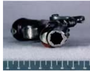
Figure 4. Muzzle view of the Deringer pistol showing the 7-groove rifling pattern. Click for enlarged image.
